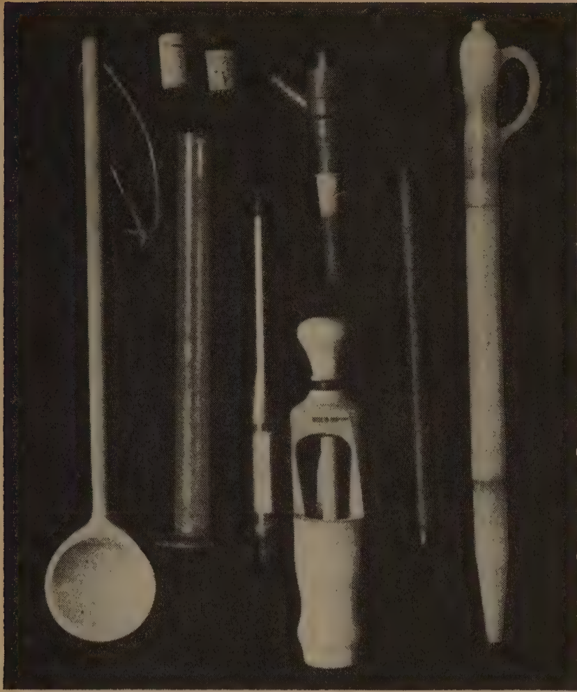
Stirring spoon, hydrometer jar and hydrometer, wine corker (lower center), wine thieves (right) and corks. Object in upper center is a convenient gadget for filling the bottles. A plastic hose is attached, and the wine bottle will be filled by siphoning to the proper level.
